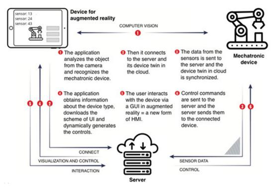
Figure 2. Proposal of a monitoring system using augmented reality. Source: [4]
