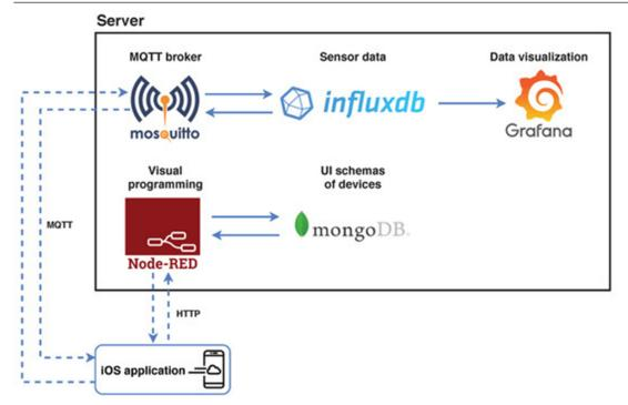
Figure 1. Server part of the solution. Source: [4]
